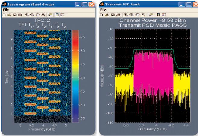
While most radio transmissions are high power density with narrow bandwidth, Ultra Wide Band (UWB) transmitters use low power density with ultra wide bandwidth. This presents unique challenges to designers of UWB devices who must trigger, acquire and analyze the single-shot, coherent waveform. Whether engineers are designing and integrating UWB radios, chirp radar, or WiMedia UWB devices into consumer, military, or computer systems, several challenges arise:
